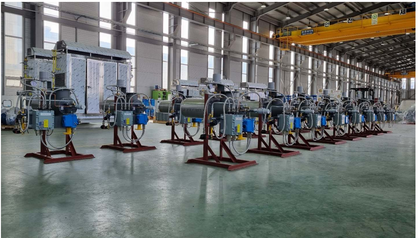
OPLE-70 Low Nox Burner / Pre-Assembled
