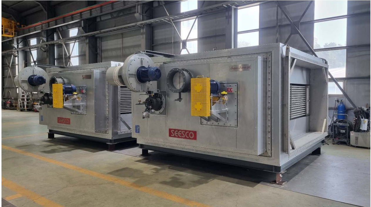
1,300 KW “Super Saver 90” In-Direct Air Heater (Food Dryer)
